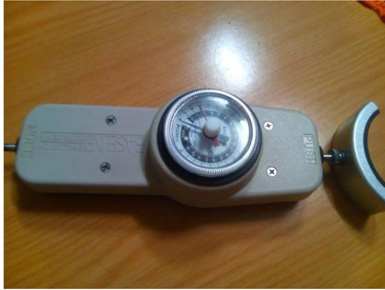
Imagen. 1 Baseline® Hydraulic Push-Pull Dynamometer
